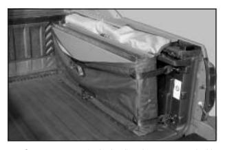
4. Store cargo panel 3 by loading the cargo panel with latches at the top of the bag and facing toward you.
